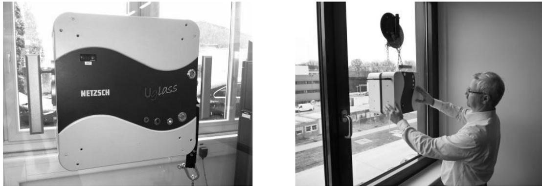
Figure 2: First prototype of the  $U_g$ -value sensor (left) and field test with anti-fall guard (right).
